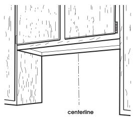
Determine and clearly mark a vertical centerline in the cabinet opening.
